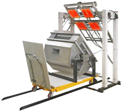
Above: Test apparatus for EN TS1187 Test 4 - Two Stages incorporating Burning Brands, Wind and Supplementary Radiant Heat, as shown in a 45° incline position. Image used with permission of Fire Testing Technology Ltd.
