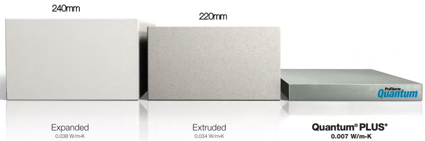
The depth of board to achieve an R-value of 6,250m 2 K/W – rounded up to the nearest standard depth.
