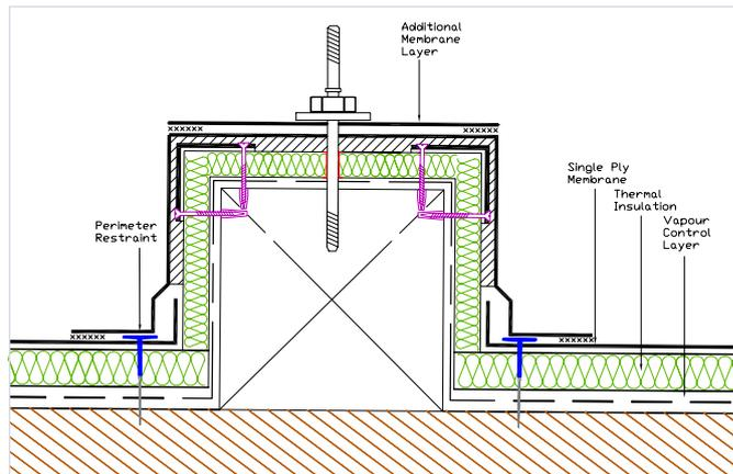
Detail 5 Load-bearing plinth for plant - principles
