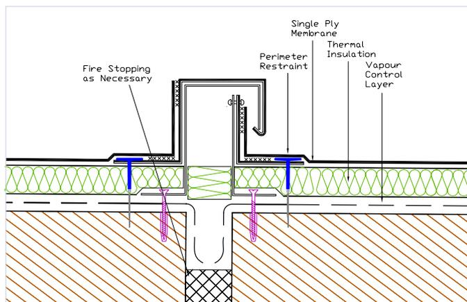
Detail 4 Movement joint – weatherproof - principles
