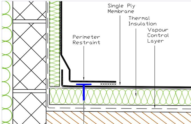
Fig.11 Restraint of membrane by mechanical fastening at perimeter (example)
