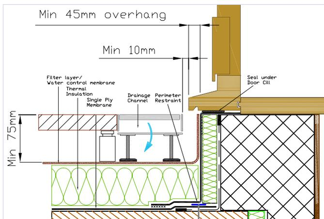
Detail 7 Level threshold – inverted warm roof - principles
