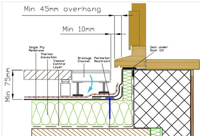
Detail 6 Level threshold – warm roof – principles
